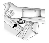
The glove box is air conditioned and can be used to store items at a lower temperature. The vehicle air conditioning must be turned on for the maximum cool air to enter the glove box. Move the slide control across the small hole to turn the cool air flow off. Close the opening to keep cold air from entering the vehicle.
